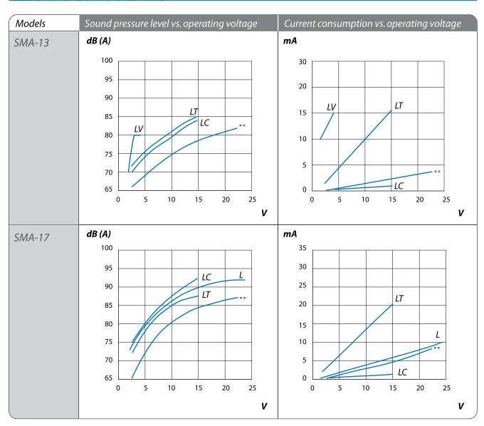
All measurements are made @ 30 cm in free air @ 21°C.
