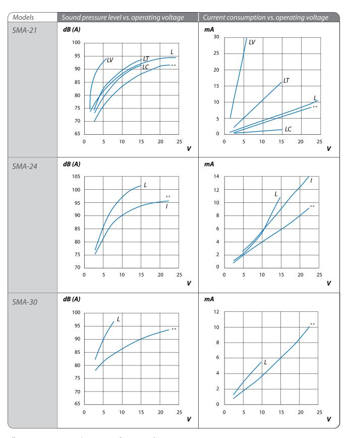
All measurements are made @ 30 cm in free air @ 21°C. °°: standard versions, respectively SMA-21, SMA-24, SMA-30.
